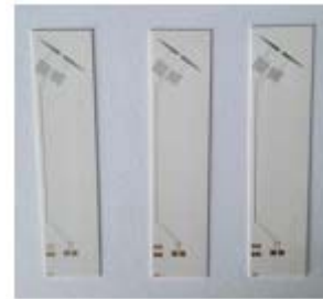
Fig. 4 Photograph of the 100MHz~60GHz dipole
